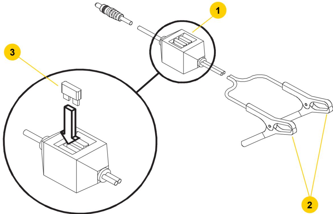
1. Battery power cable 3-amp fuse box
