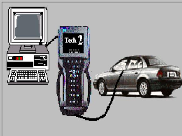
Verify vehicle battery fully charged, engine off, ignition on
