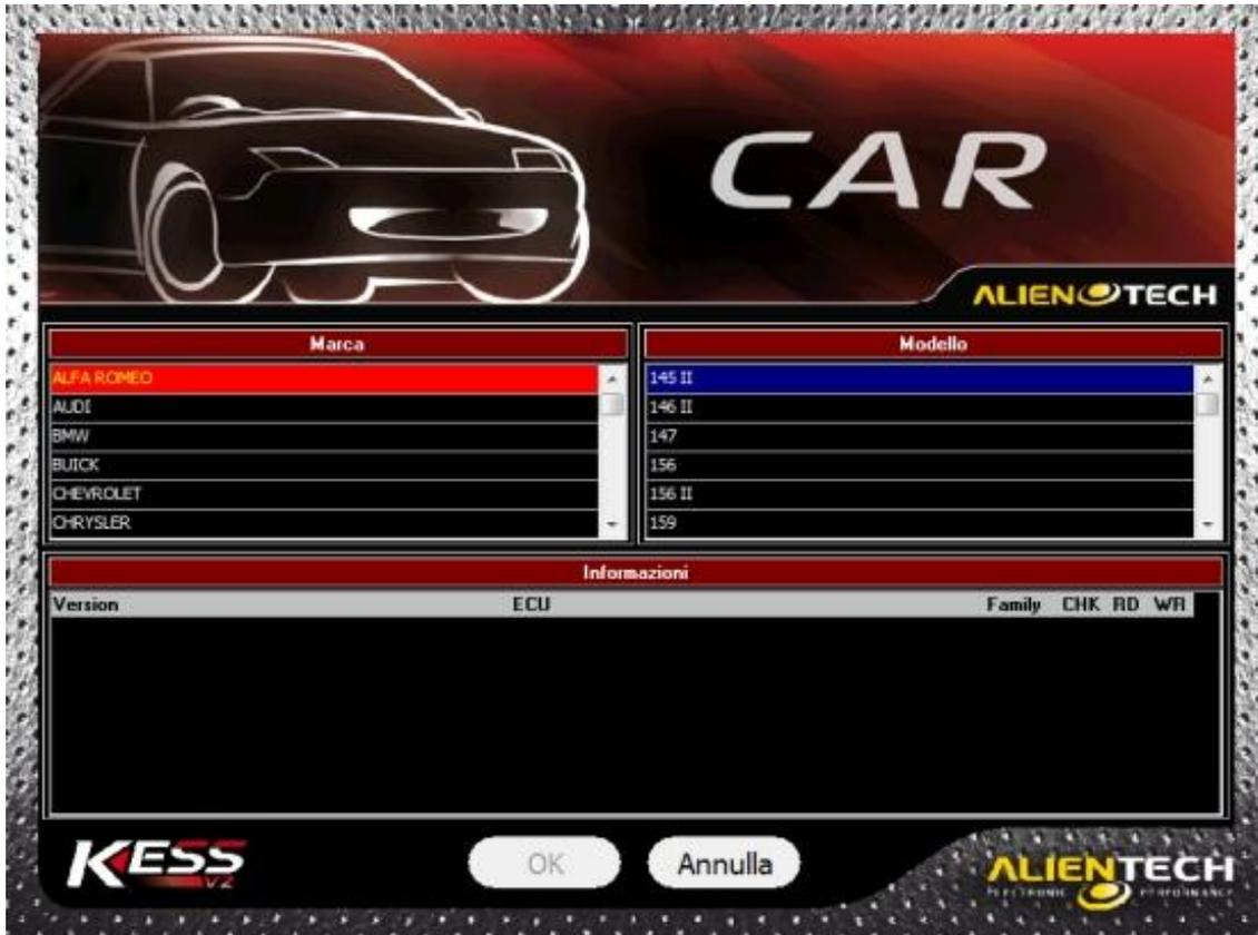
The window with every kind of vehicle displays: brand, model and the version of the ECU related to the engine equipped on the vehicle. On the right side there are three checkboxes that indicate what KESSV2 can do: Checksum (CHK), Reading (RD), Writing (WR).
