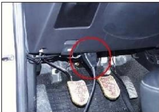
-Location of OBD-II diagnostic connector-
