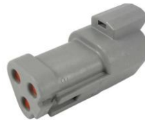
Figure D2 Image of J1939 Terminating Resistor on J1939-11 Network (Twisted Shielded Pair)
